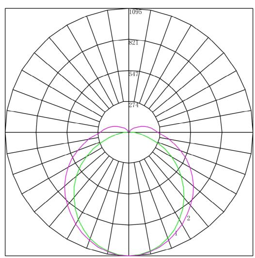
Maximum Candela = 1094.783 Located At Horizontal Angle = 0, Vertical Angle = 0 # 1 - Vertical Plane Through Horizontal Angles (0 - 180) # 2 - Vertical Plane Through Horizontal Angles (90 - 270)
