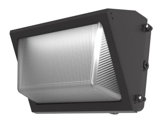
The OW Series Wall Packs feature a rugged die-cast aluminum housing available in 3 different sizes for a fully scalable solution. The fully gasketed housing is IP65 rated for whole luminaire ingress protection against moisture and environmental contaminants.
